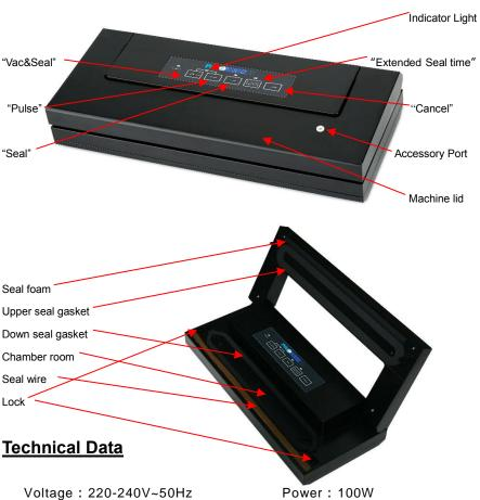
Pressure: -21"Hg/-711mbar(±5%) (directly in pump
